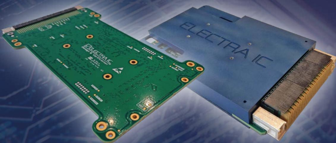
The BitFlex-VPX3-MZQU is a high-performance FPGA processing module based on the Xilinx Zynq UltraScale + family of FPGAs. It provides multiple high-speed fabric interfaces, external memory, an FMC site, and high-density I/O. It is ideal for customizable, high-bandwidth, signal-processing and image-processing applications.
