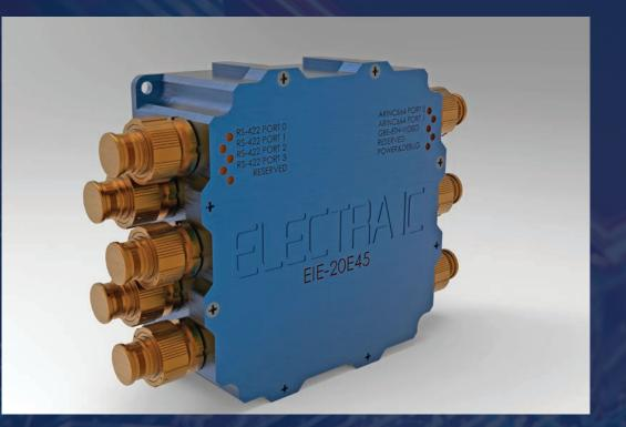
ARINC664 End System Equipment implements ARINC664 part 7 and provides interface between aircraft LRUs and ARINC664 network. It offers an adaptation between RS-422/ARINC664 and Ethernet/ARINC664. In this manner, four RS-422 ports and one Ethernet port are added to the design such that an easy adaptation can be done when a customer wants to use LRUs with flight heritage. Equipment also has a test mode that measures the latency occurred on messages of the relevant VL number.
