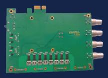
The Avionics Interface Converter is a versatile interface card designed for testing avionics interfaces. It supports MIL-STD-1553 and ARINC-664 communication protocols. This board facilitates the integration and data communication of avionics systems, offering the high reliability of the 1553 bus and the fast data transmission of the A664 Ethernet-based protocol.
