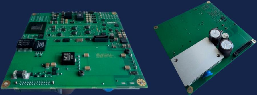
The BitFlex-SPB-A7, an advanced hardware design platform centered around the powerful Xilinx Artix-7 FPGA. This cutting-edge board boasts high-performance capabilities and a comprehensive set of peripherals, including Ethernet, RS422/RS485, and high-speed DDR3 memory.
