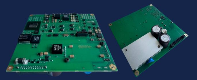
The BitFlex-SPB-A7, an advanced hardware design platform centered around the powerful Xilinx Artix-7 FPGA. This cutting-edge board boasts high-performance capabilities and a comprehensive set of peripherals, including Ethernet, RS422/RS485, and high-speed DDR3 memory.
