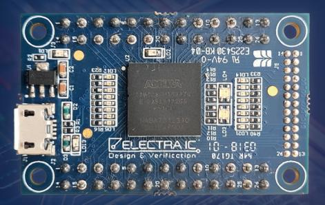
The Flexy FPGA board is a low-cost, open-source FPGA board in a tiny form factor. Solder on pins for use in a breadboard or PCB socket; or solder connectors, wires, and components directly onto the board.
