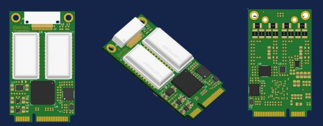
This Full-Mini Card Form Factor F2 PCIe board allows two dual redundant MIL-STD-1553 channels to be easily added to any small embedded system to provide a cost-effective, lightweight, small-size, rugged and reliable 1553 bus interface. The board can meet rugged levels of shock and vibration along with a maximum temperature range of -40°C to +85°C.
